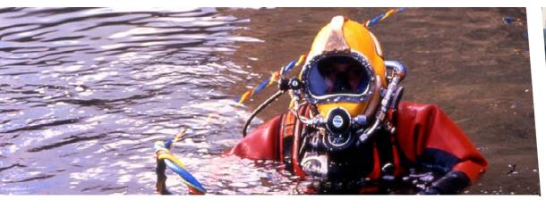
The "Dirty Harry" Contaminated Water Diving System is designed to provide a safe and efficient surface supplied system which minimises the risk of contact between the diver and the water in which he is diving.
