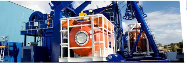
Divex Modular Saturation Diving Systems are designed to be rapidly deployable and flexible to allow rapid configuration on a variety of vessels.
